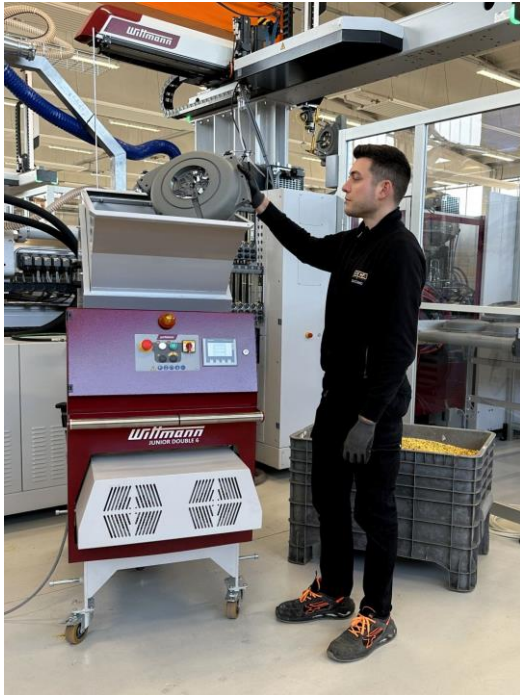
Sprue and reject parts are reground directly next to the machine. For many products, the granulate can be blended in with the virgin raw material. (Photo: WITTMANN)
